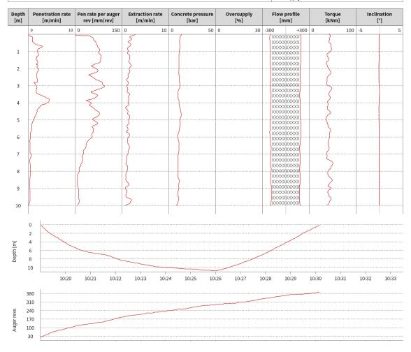
The individual, pile specific reports for MOVAX MPL CFA include the following information: Position data, Pile type, Pile dimensions, Pile depth, Angle, Torque, Concrete volume, Concrete pressure, Start time, End time, Elapsed time, Date
