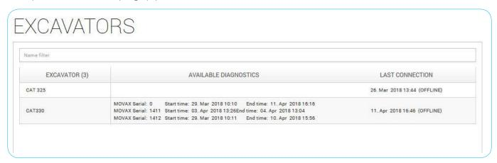
After the carrier is selected, the diagnostics tool will show the time periods for which the detailed data is available. The selected time interval can be downloaded by choosing the start time and duration and by pressing the 'Activate range' button.
